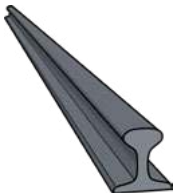
rail: guides the train's wheels
