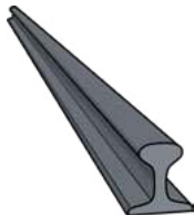
rail: guides the train's wheels
